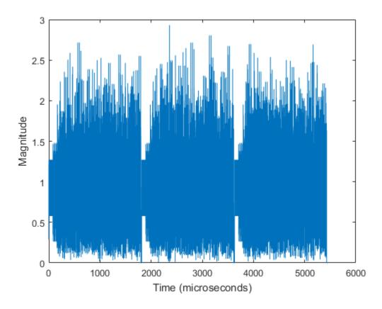
The plot shows three S1G format packets, with each packet separated by 15 microseconds of idle time.
