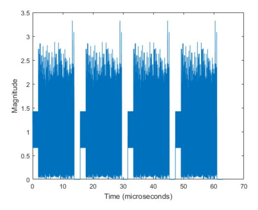
The plot shows four DMG format packets, with each packet separated by 2 microseconds of idle time.
