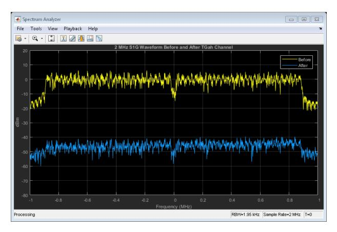
Path loss accounts for the roughly 50 dB of separation between the waveform before and after it passes through the TGah channel. The path loss results from the default transmitter-to-receiver distance of 3 meters, and from shadowing effects. The signal level variation shows the frequency selectivity of the delay profile across the frequency spectrum.
