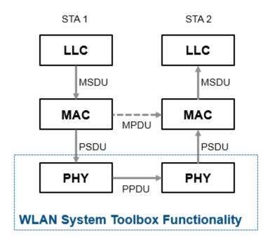
WLAN System Toolbox functionality focuses on PHY implementations and the exchange of PPDUs between PHY peers. Messages exchanged between protocol stack layers are briefly described here. For more information on these messages, see IEEE Std 802.11-2012 [2].
