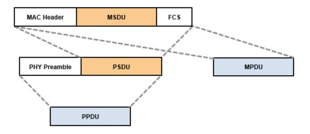
**Note:** In reference to PSDU, the terms PLCP SDU and PHY SDU appear in the 802.11 standard. PLCP is the physical layer convergence procedure sublayer of the PHY. No distinction is made when the terms are used between layers.
