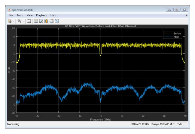
Path loss accounts for the roughly 50 to 60 dB of separation between the waveform before and after it passes through the TGac channel. The path loss results from the default transmitter-to-receiver distance of 3 meters, and from shadowing effects. The signal
