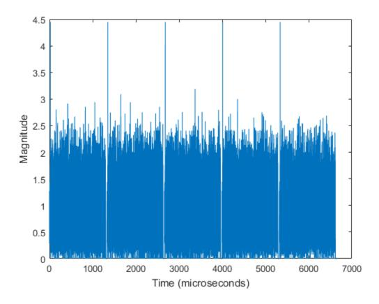
The plot shows five HT format packets, with 30 microseconds of idle time separating each packet.
